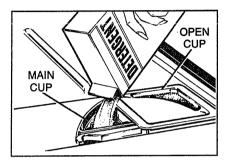
See "Detergent Usage Guide" below. (Be sure the Cycle Indicator Dial is at OFF position before adding detergent.)
